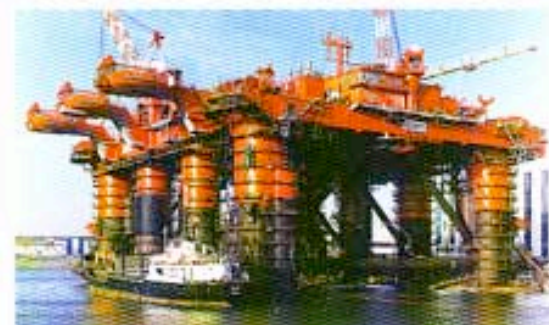
Semi-submersible 500 man accommodation platform built for Norway in 1983 by Alsthom at Saint Nazaire.
